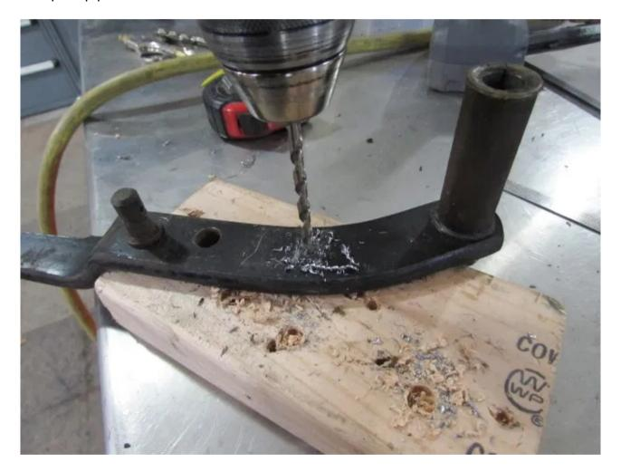
On this 1965 Mustang, the factory clutch pedal is very close to the fulcrum, yielding a suitable ratio for the master cylinder. We were even able to use the original firewall hole.
