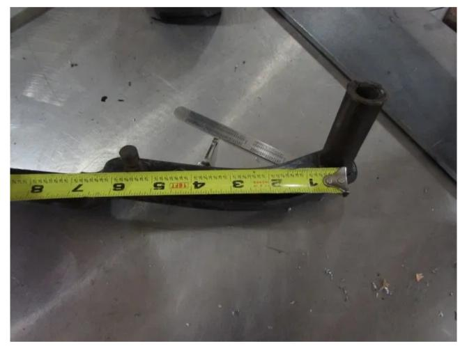
The pedal measures 14 inches from the fulcrum to the center of the pedal. The math reveals this is a 2.48:1 ratio, which is ludicrously low.
